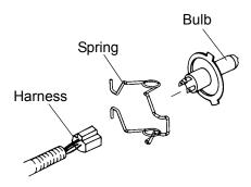
5. Grasp the bulb by its metal base and carefully separate the bulb from the harness.
